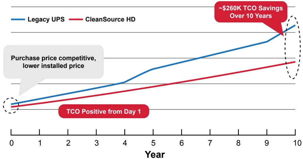
Figure 5. TCO comparison between CleanSource HD UPS and a legacy UPS. Assumptions: 1 MW load with 2N design; CleanSource 750HD: 96% efficient; legacy UPS: 94% efficient, 6 minute VRLA batteries w/ 5 year replacement cycle; \$0.10/kWh energy cost
