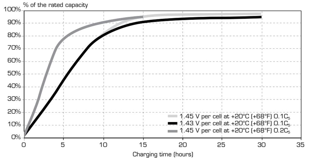
*\*For charging voltages higher than 1.45 V/cell, a current limit of 0.1 C<sub>5</sub>A is recommended*
