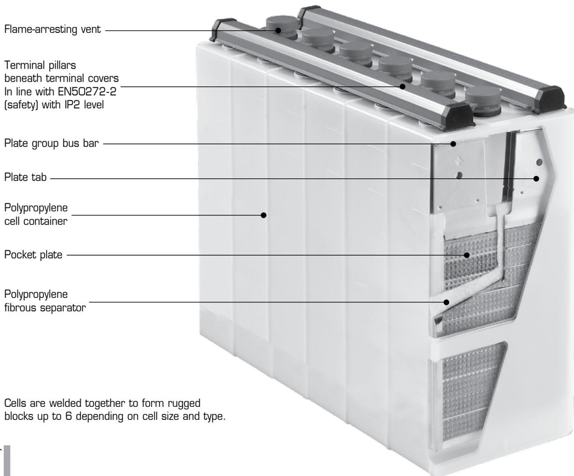
Cells are welded together to form rugged blocks up to 6 depending on cell size and type.
