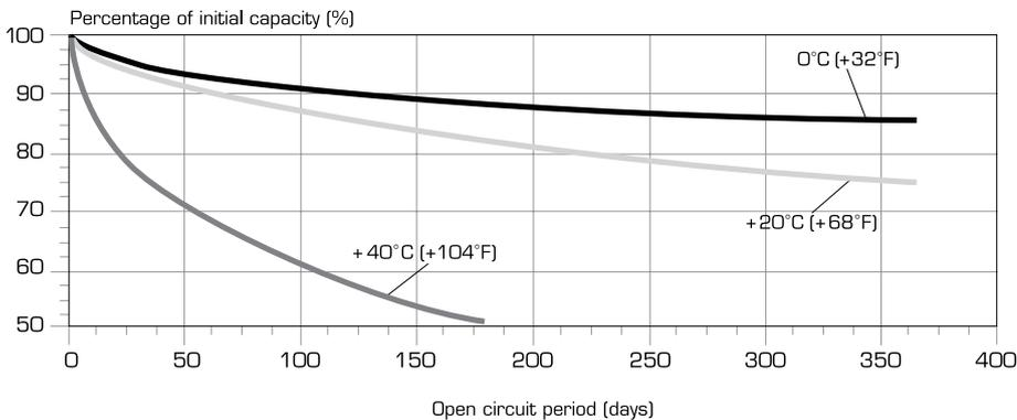
Figure 2: Typical open circuit loss variation with time.
